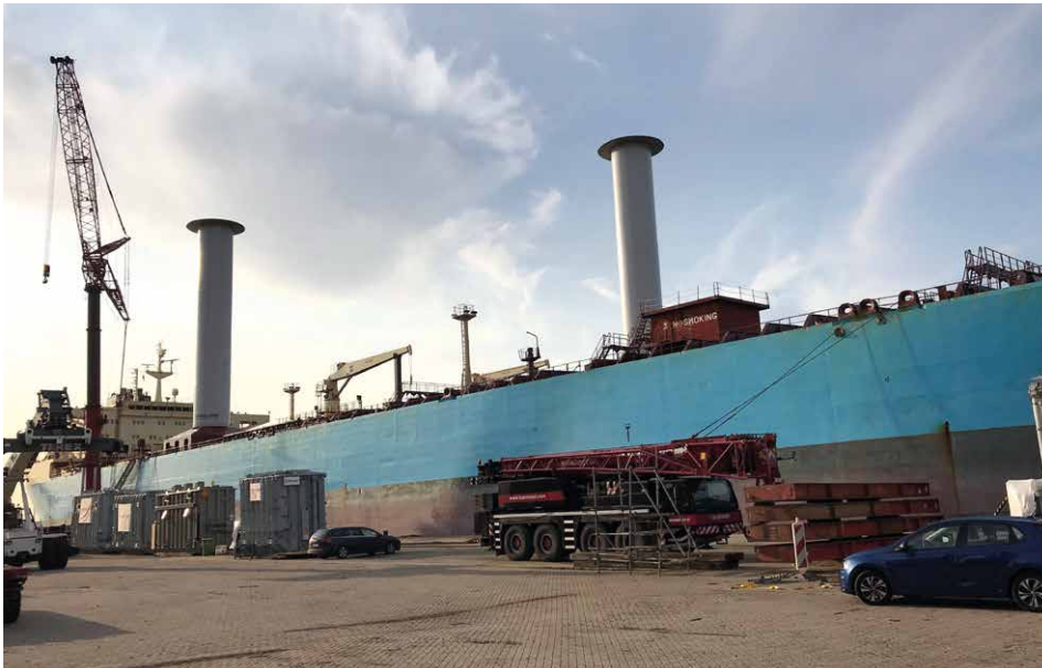
The Rotor Sails seen being fitted in Rotterdam
