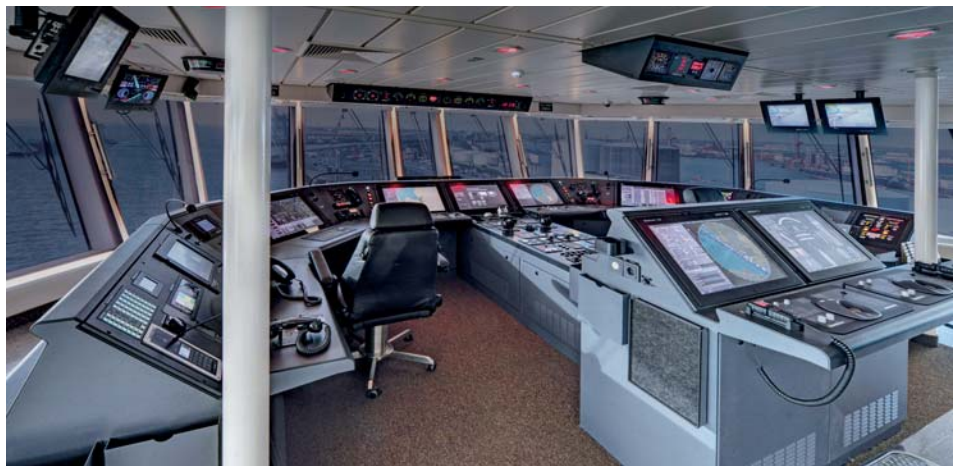
A SAM Electronics NACOS Platinum navigation automation control assembly embodying functionally integrated human machine interface (HMI) design principles.
