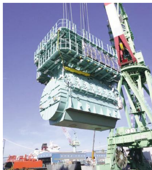
MDT's ME-LGI engine being lifted into place.
