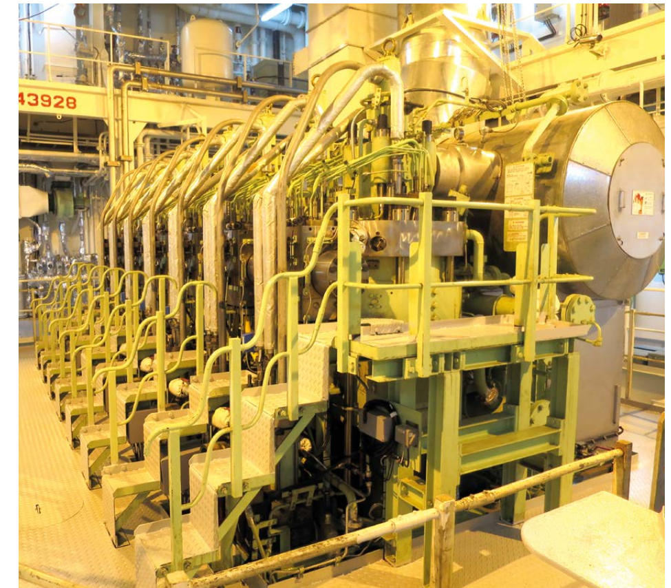
The gas driven 7G50ME-GIE engine
