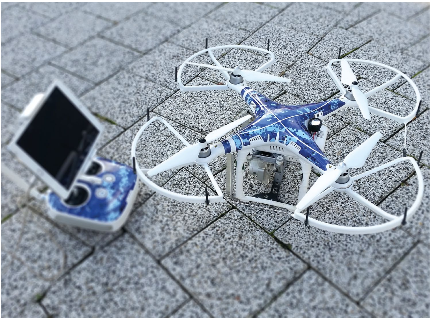
DJI Phantom: The DJI Phantom drone can operate for about 20 mins and is lighter than the Custom drone. It is used for external surveys but can also be flown inside spaces, such as tanks. When fitted with its protective shield it is more resistant to damage.
