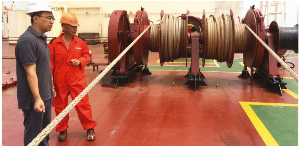
After six years of operation, DSM Dyneema ropes were said to be good for 10 years service
