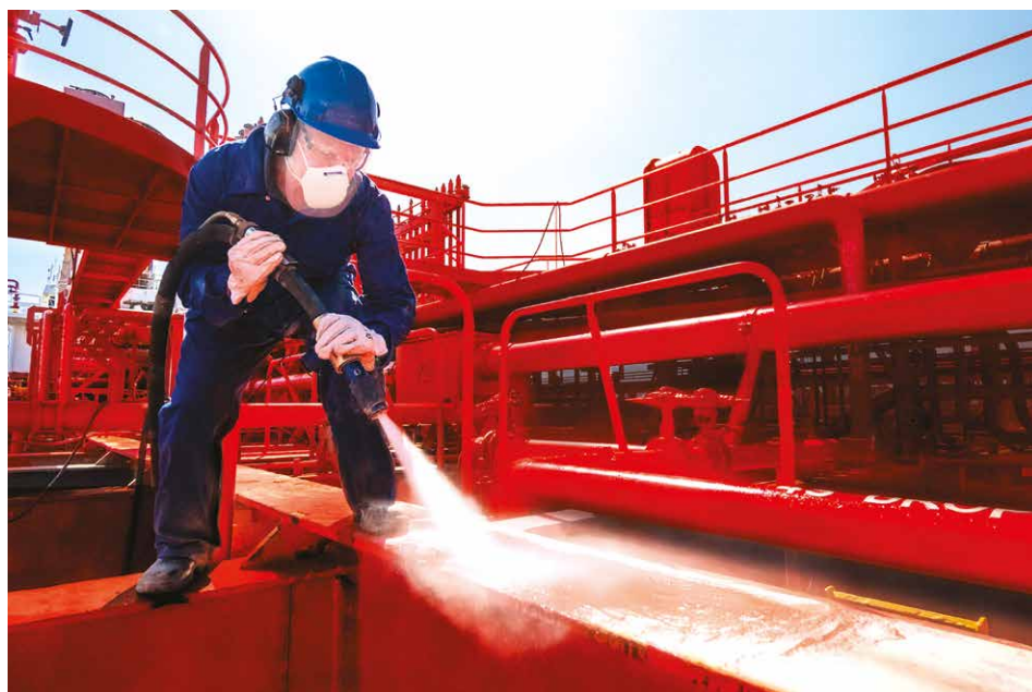
Surface preparation is as good as dry blasting
